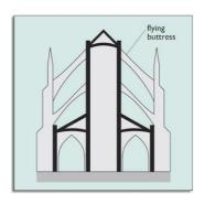
Flying buttresses are external arches that are high up on the cathedral. They support the walls and prevent the problem of outward thrust.
