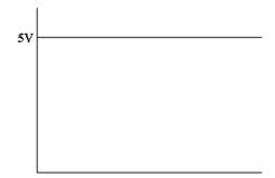
In order to work correctly the PICAXE 18X must have a continuous steady 5 volt supply. There are two main things that might affect the circuit and cause further problems.
