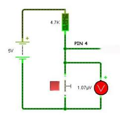
When the switch is pressed the voltage drops to a value very close to OV. This is what we should expect to happen. In this case we say the PIC sees the value on Pin 4 as a O.
