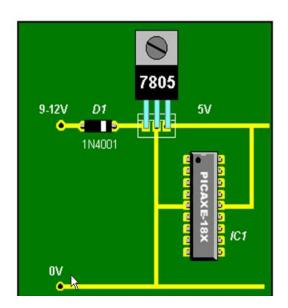
This arrangement uses a mains operated 9-12 volt power supply. A 7805 voltage regulator reduces the voltage to a suitable 5 volts. A diode is included to ensure the power is not connected the wrong way around to the circuit thus damaging some of the components. Pin 5 is connected to OV and pin 14
