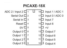
Remember that the PIC has 8 outputs, pin 6 through to 13. These outputs are forced high and low by setting them using appropriate software.
