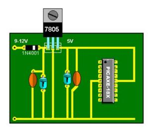
To overcome this problem we use two  $0.1\mu F$  capacitors which filter out any unwanted noise from the circuit. This filtering works on the basis that capacitors block DC but allow AC (noise) to pass through. The
