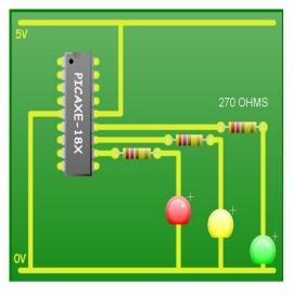
The circuit used to turn LEDs on and off is relatively simple. Since LEDs only require a small current (10mA) to operate then we can connect these components directly to the PIC. Note however that this is the exception rather than the rule. As it can only source or give out a small current, the only other device that can be switched directly is a piezo buzzer/sounder.
