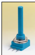
Variable resistor & symbol
